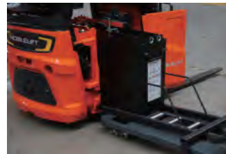
Battery compartment with fork pockets for 16N.
