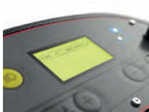
LCD heads-up display incl. hour meter
