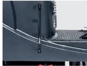
Water solution level indicator with volume visible on the tank
